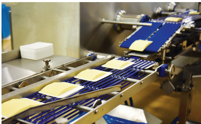
On the new packaging line, up to 80 packages per minute, are automatically sliced, packed and inspected
