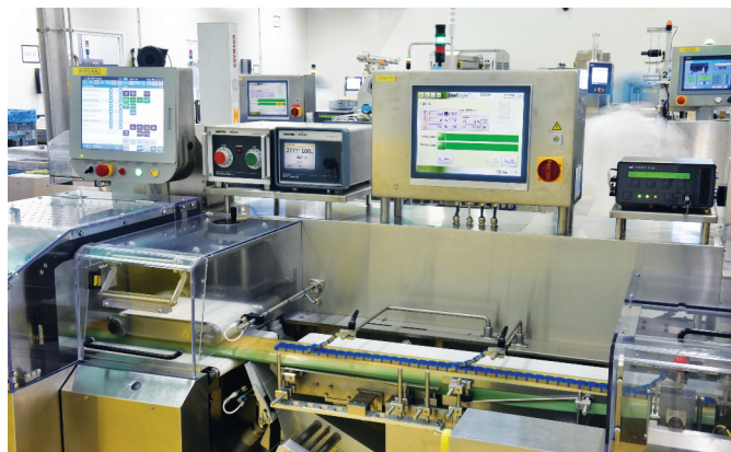
Also the new OMORI flow-pack line is equipped with the SealScope™ seal inspection system. In the background one can see the first installed SealScope system
