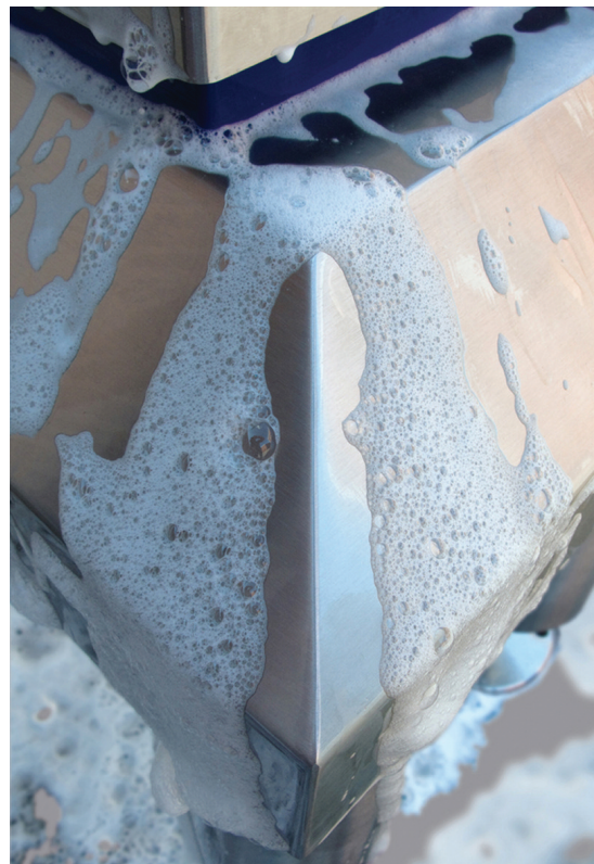
Look for smooth, crevice-free contact surfaces to reduce the risk of cleaning agents not being fully rinsed away.
