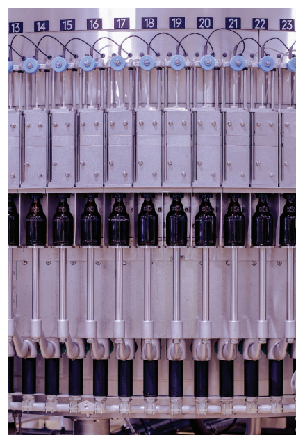
During bottle filling a new hollow probe filler enables greatly reduced CO 2 consumption on the one hand and even lower oxygen pickup on the other
