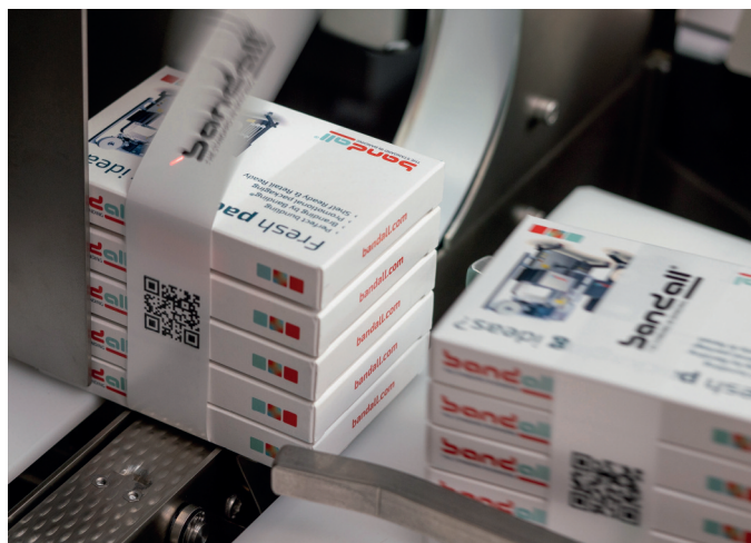
Implementing OMRON's optical sensor and a digital fiber amplifier in Bandall's stand-alone banding machines has enabled creating a single solution for meeting various needs.
