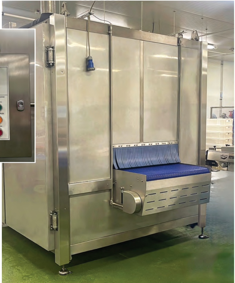
Equipped with a Siemens controller, belt speed can be finely tuned to suit the product
