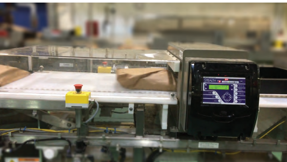
Halo Automatic Testing can validate the performance of metal detectors by testing three metal samples - ferrous, non-ferrous, and stainless steel - sometimes in multiple positions, without interrupting production.
