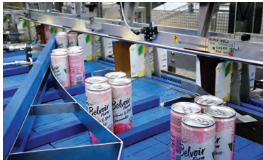
The Automatic Beverage Multipack Machine cartons small, slim and wide 150ml, 250ml, 330ml cans into numerous pack sizes
