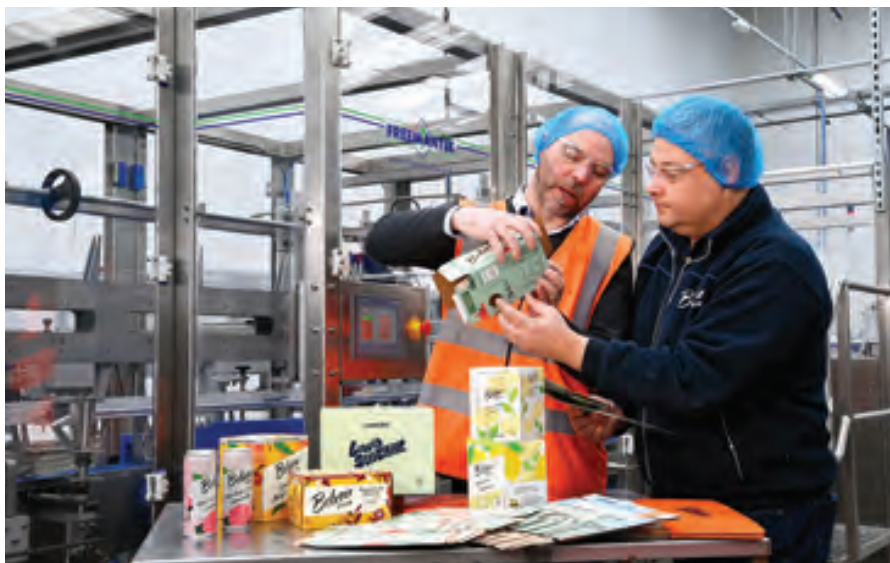
Belvoir's Martin Reynolds (right) The T. Freemantle Machine easily and consistently runs at 55 to 70 cartons per minute.
