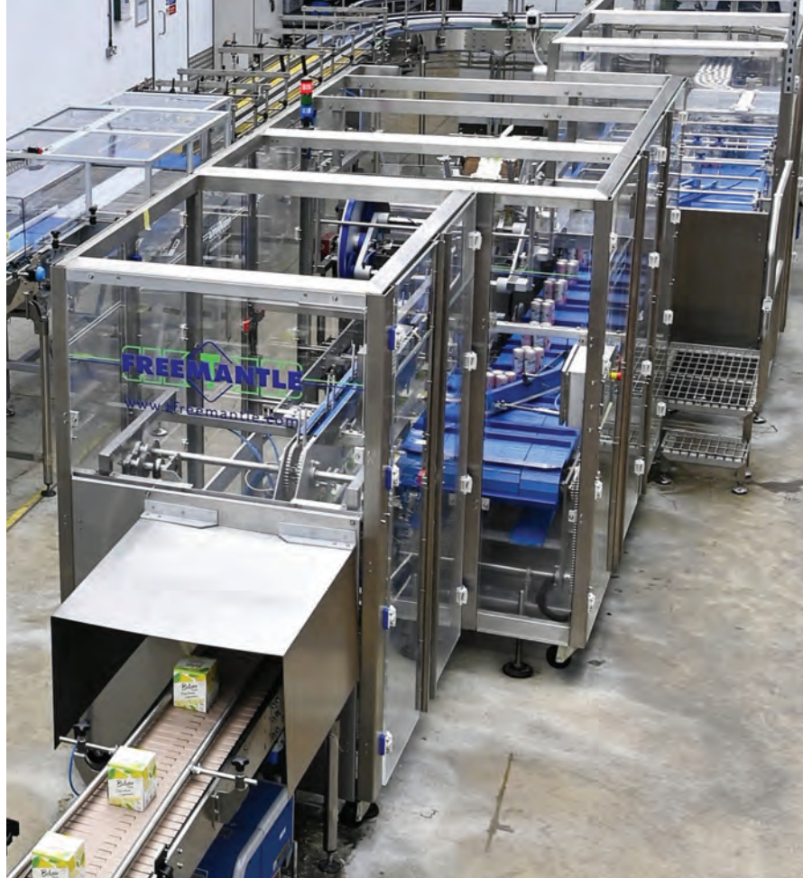
T. Freemantle ultra-clean open frame Automatic Beverage Multipack Machine_4X faster cleaning and maintenance
